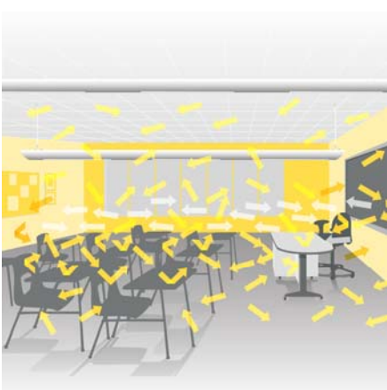
Figure 2. Sound field at steady state in a room with suspended ceiling and sound scattering objects.
