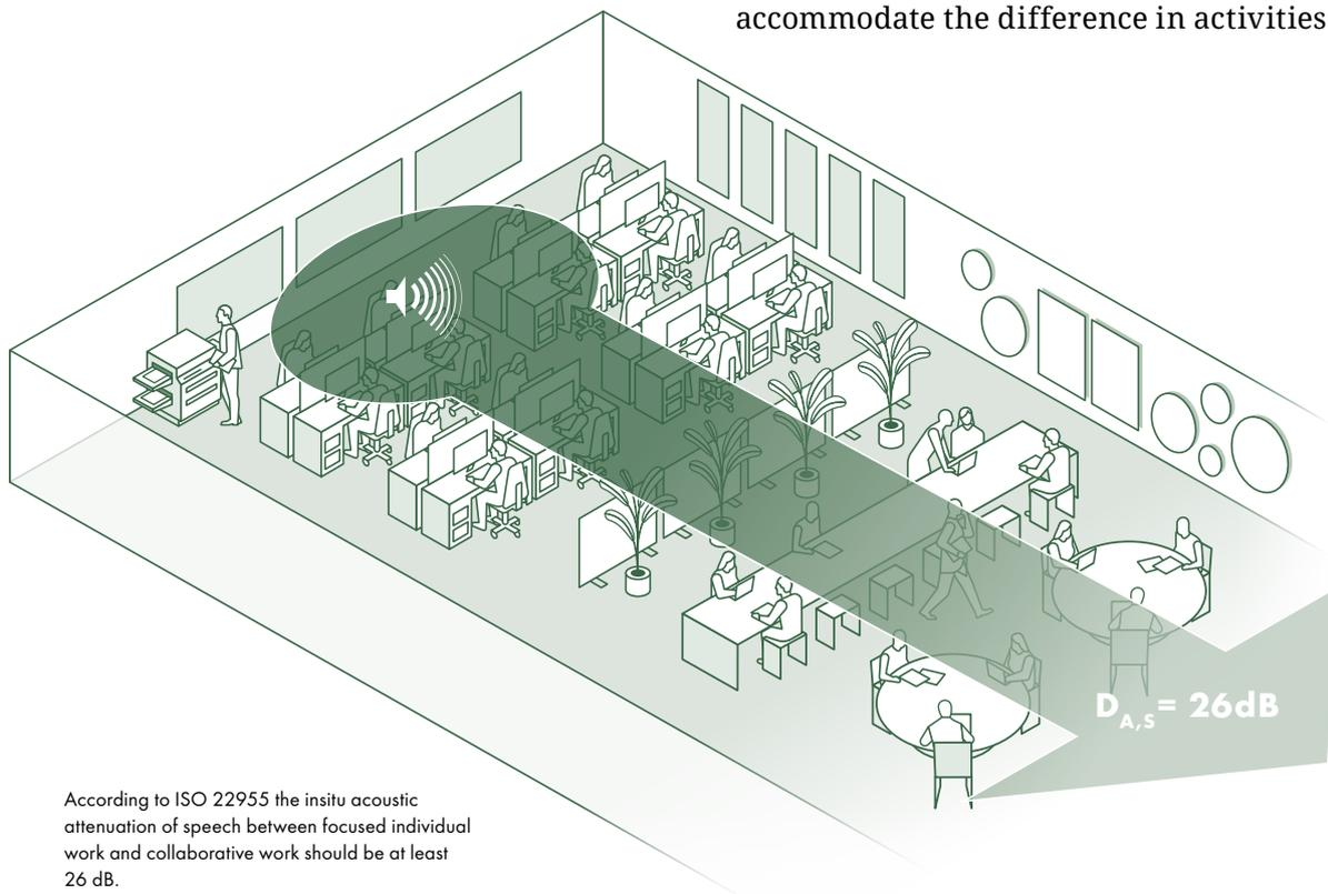
According to ISO 22955 the insitu acoustic attenuation of speech between focused individual work and collaborative work should be at least 26 dB.
