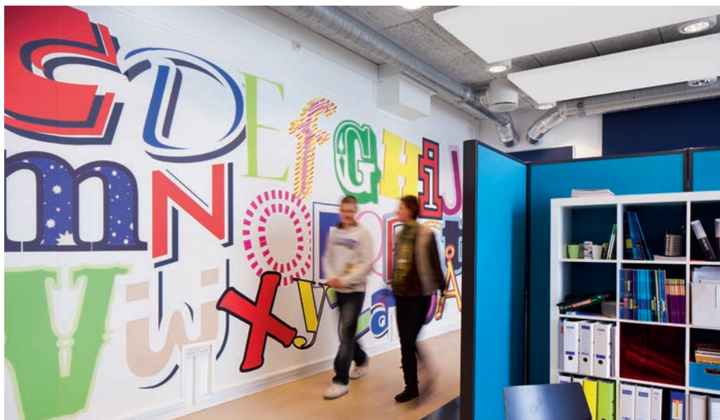
As requested by the teachers, the wall absorbers in the two rooms have cheerful, colourful designs. The surfaces of the wall absorbers and the sound absorbing screens are hardwearing and can also be used as noticeboards.
