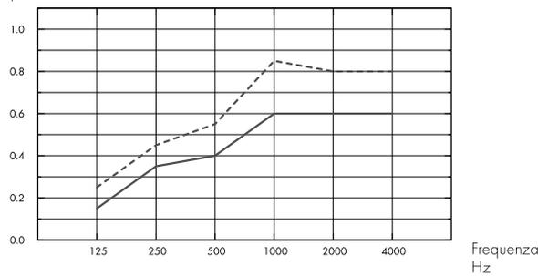
— Solo Baffle ZigZag 1800x300/200, spacing 600, direct mounting
