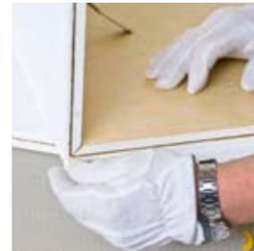
Reinforcing plug A plastic reinforcing plug is installed at the joint to give the vertical surface a clean appearance.
