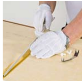
Reinforcing the fold A concealed aluminium rod reinforces the fold. This provides a solution with good resistance to impact and knocks.
