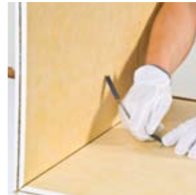
Accurate angles The Connect Hook ensures an accurate 90° angle.
