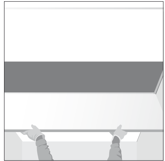
During fitting, the ceiling panel is pressed against the spring inside the profile and is held in place by the channel.
